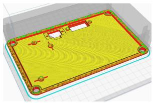
The pipeline for prototyping a part begins with an engineer creating a 3D part in software. But from there, additive manufacturing has greatly streamlined the process. Entire sets of 2D drawings detailing specifics about the parts to be produced, as well as tooling, can usually be bypassed entirely if the part is to be printed.
