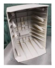
The part was cleaned off and could then immediately be tested and evaluated just like a production speaker. Testing found that there were improvements to be made, and thanks to our ability to do the 3D printing in-house, these changes could be almost immediately tested.
