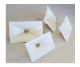
The parts in this case were ready the next day, but production time can vary from a few hours to several days, depending on size. Because the waveguide contains many small features, it was printed on a Stratasys polyjet printer, which uses a hybrid technology between FDM and resin printing to produce very smooth surfaces at high resolution.
